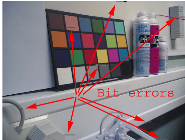
Figure 93 Bit errors caused by JPEG compression
