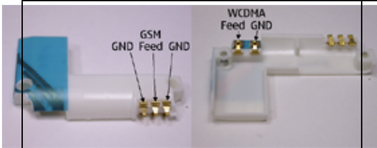
Figure 67 Antenna frame, contact springs and WCDMA antenna
