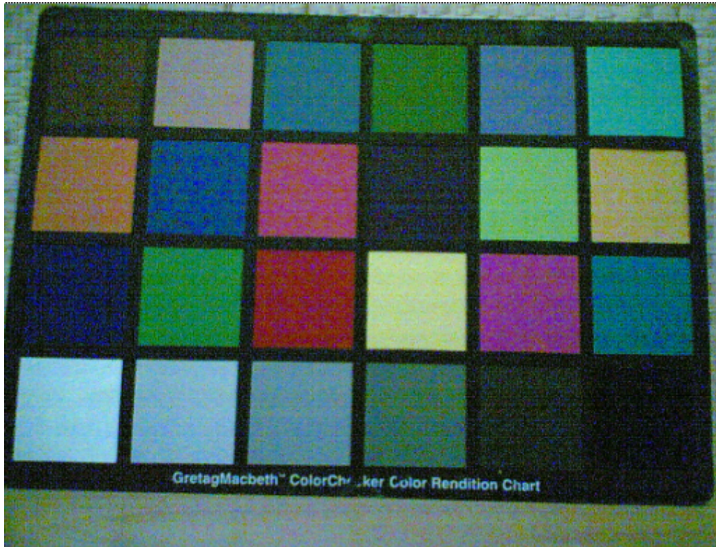
Figure 82 Noisy image taken in +70 degrees Celsius
