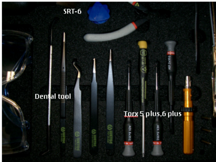
Figure 41 Required tools for RM-42 disassembly / reassembly
