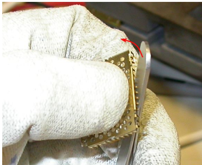
Figure 76 Squeezing the sides of the shield lid
