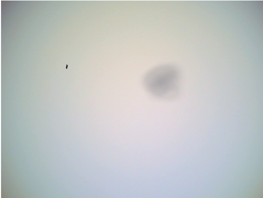
Figure 88 Effects of dust on optical path
