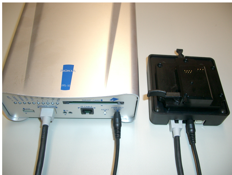
Figure 39 CU-4 flash concept with FPS-10
